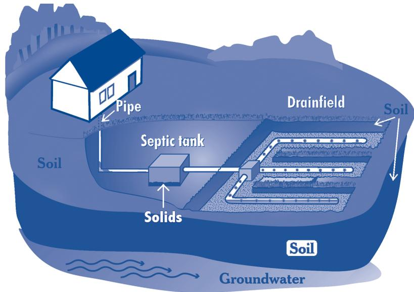
In some situations, effluent from a septic tank will not be dispersed to a traditional drainfield. Alternative systems in use today include sand filters, mounds, wetlands, gravel-less drainfields, pressure dosing, and aerobic units. Servicing requirements for these systems vary and should be obtained from your local sanitarian or septic system contractor.
